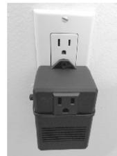
16. Now it is time to plug-in your garage door opener's power cord, except this time it will plug into the SureLock control module you just installed.
